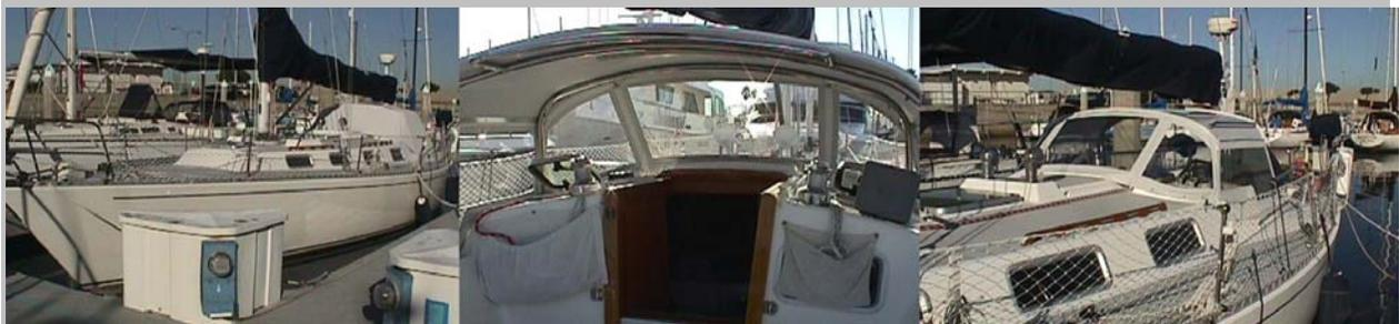
This dodger has a fiberglass top and removeable Lexan windows. It is entirely self-supporting with 1 1/8" SS bows, yet can be totally removed from the mounting sockets quickly by removing set screws. Good handholds at sides and back, and all the windows remove easily for ventilation. We even added a boltrope and track to mount our awning to the back of the dodger.
