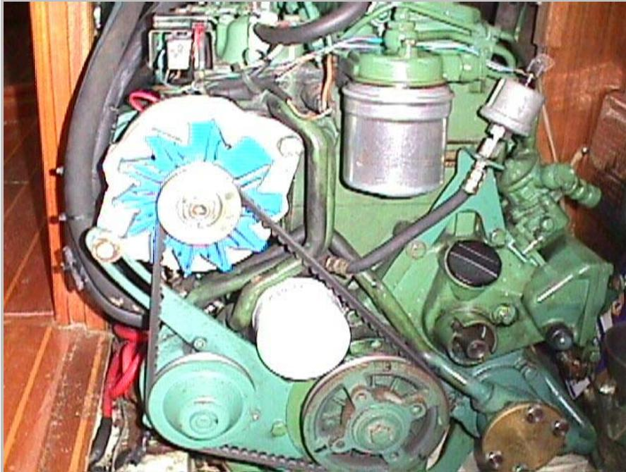
We finally refurbished the injectors as we got close to 2000 hours on the engine. We also found it to be a good idea to have the exhaust elbow and heat exchanger cleaned out every 3-4 years to prevent clogging. Other maintenance has just been regular oil and filter changes. We use solar panels and do not run the engine out of gear for charging, which seems to keep problems down.
