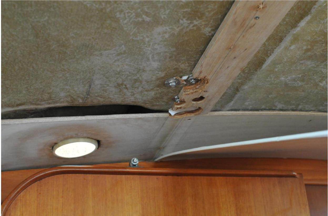
**Headliner removed, screws/nuts exposed.**
