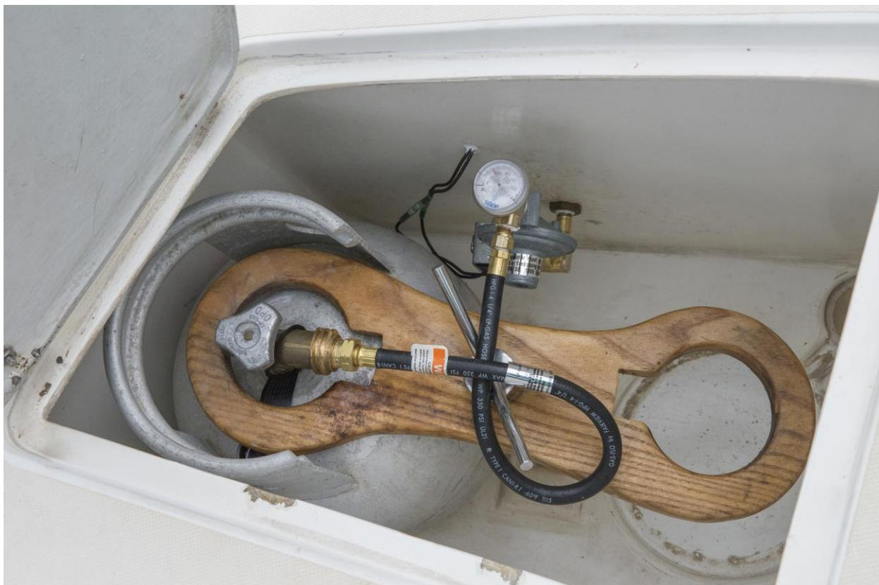
You get a good view of the components: Tank, Tank Valve, Pigtail Hose, Regulator and Gauge, Solenoid, Solenoid to Copper Tube Connector, the Compartment Vent and the Tank Tie-down.
