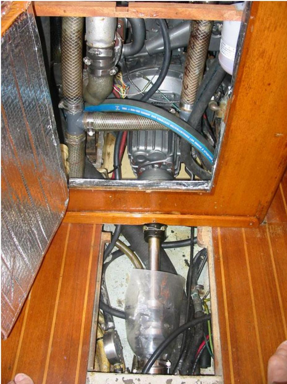
You do have to have the "high speed" model with the water injection tube otherwise water does not lubricate the cutlass bearing when the boat is under way.
