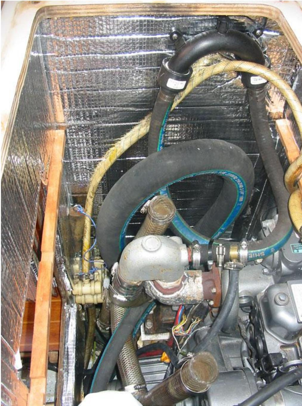
The sink doesn't even get warm now. The Perko sea water strainer (needs to be 1") is now located over the bilge so the water does not run onto the hot engine and you do not have to remove the sink to clean it. The fuel filter is now under the sink with the fresh water overflow. The only negative I have found is that it is a huge job to change a sea water impeller because it faces aft on the port side of the engine.
