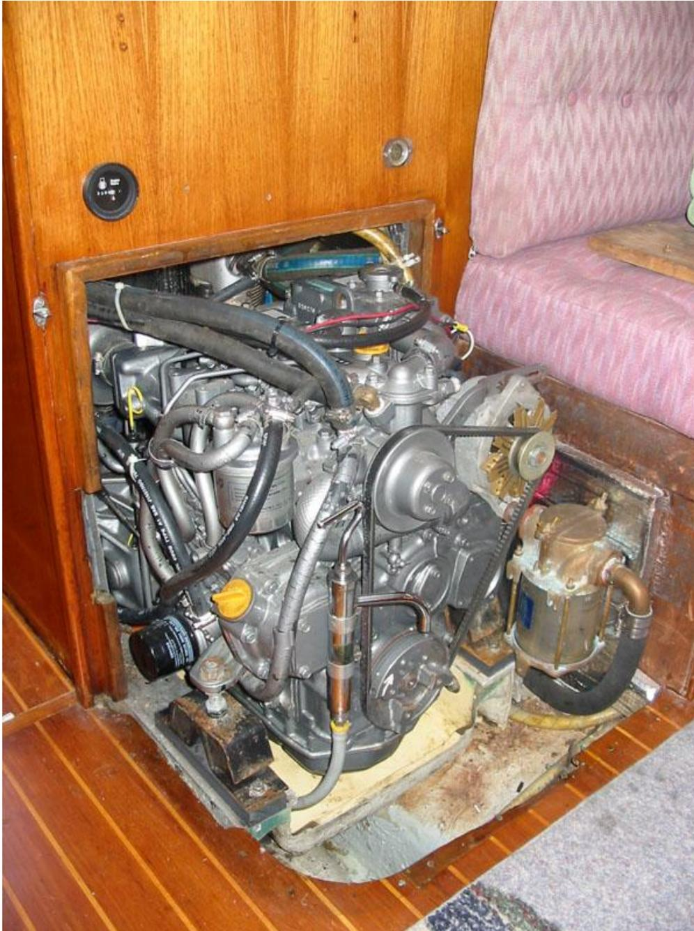
The raw water intake through hull and Perko strainer must be changed to 1" for the Yanmar (the Volvo is 3/4"). We used the original size exhaust, but replaced the hose. The original was 2 1/4" and the Yanmar calls for 2". We did not want to change the lift tank or the through hulls. We routed it the same but anchored the aft loop much tighter to prevent movement.
