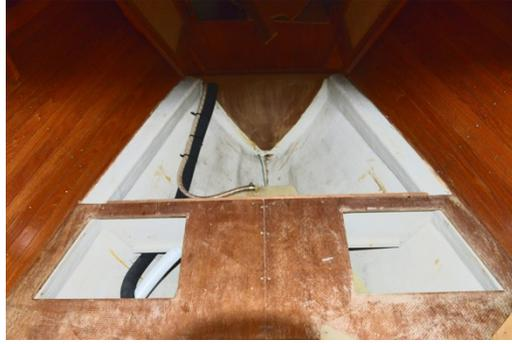
Forward panel removed, small bulkhead removed. Pumpout (black) and top vent hose visible.
