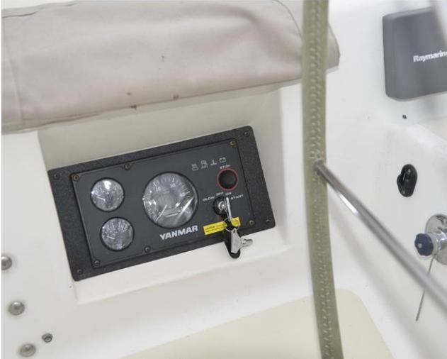
So there was an existing water temp gauge below the main panel in the nav station, not that it was doing much good there... So we'll put the fuel gauge there. Have the old one in the picture, but we'll spring for a new one for the old girl.
