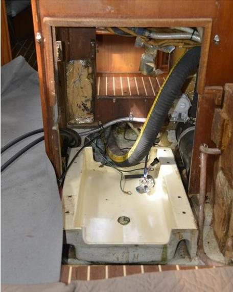
The sink drain through-hull – staying where it was, but getting replaced – time to do it. Also reorganizing the filters.
