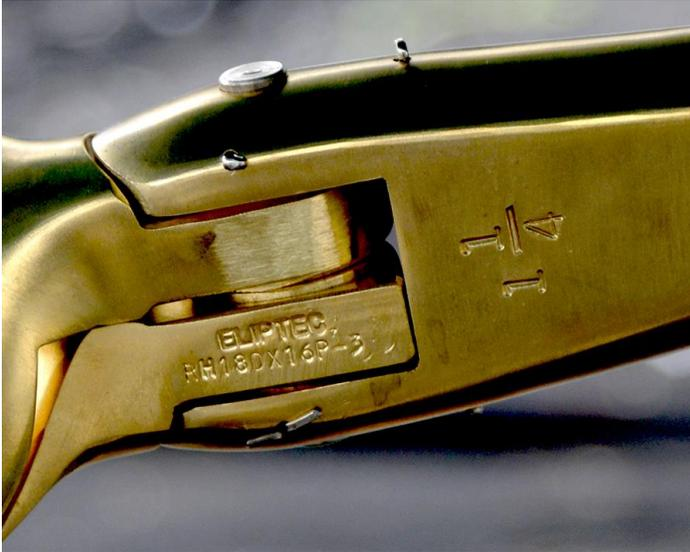
Left enough space for a kelp/line cutter if I add it in the future. On the J40, the engine is far enough forward that you can drop the shaft without pulling out the rudder – pretty easy.
