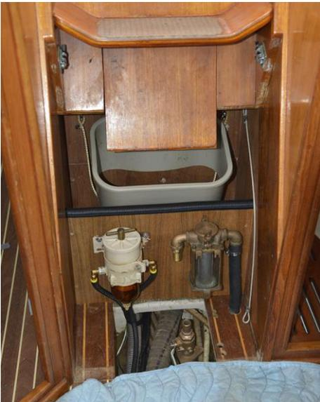
Initial Fuel Filter, directly between the tank and motor (on the left) and the water intake filter on the right. The engine intake through hull goes just forward of the little bulkhead with an opening. All very clean and easy to get to. The fuel filter used to be in the engine compartment and the Yanmar alternator sticks into the space where it used to go.
