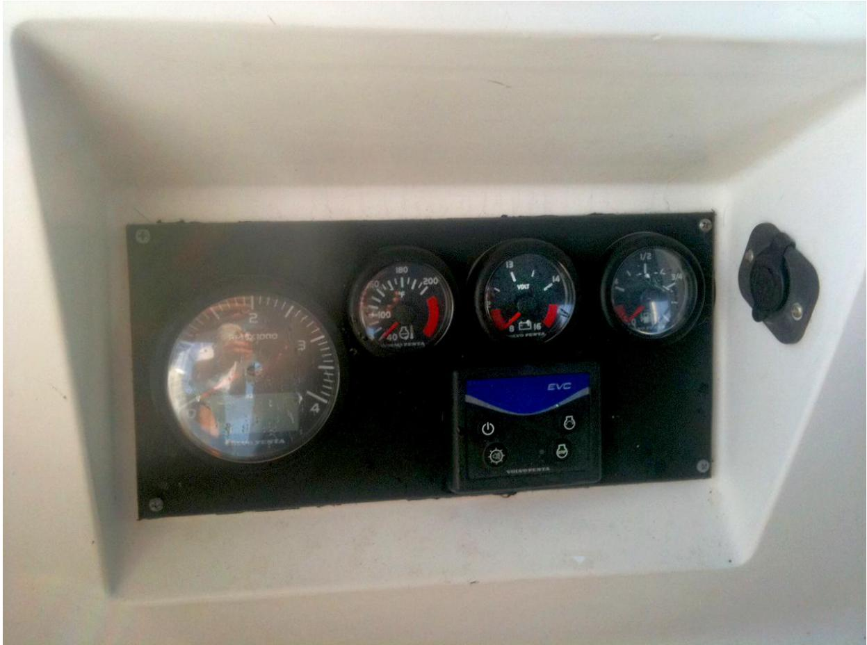
The choke, start button, and stop pull lever have been replaced with an electronic vessel control (EVC) in the D2 series installations. The LCD in the Tach provides engine hours.
