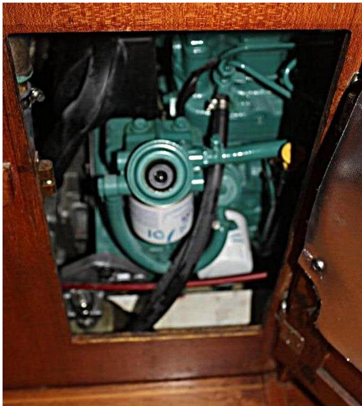
Above (sorry it's out of focus) is of the door on the starboard side of the engine compartment. You can see the fuel and oil filters, the priming pump, and the yellow dipstick. Very convenient!
